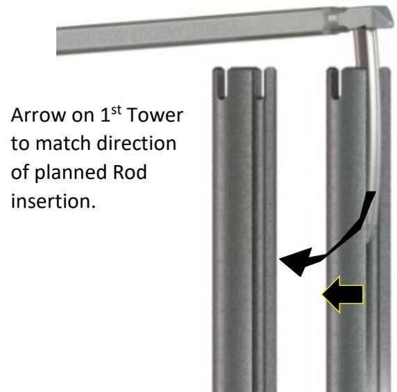
Arrow on 1<sup>st</sup> Tower to match direction of planned Rod insertion.
